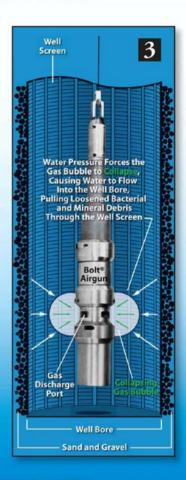
Compressed air or inert gas are the sources of AIRBURST® energy, providing you and your customers with an effective and responsible green alternative to other methods.
